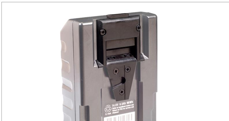
A unique feature of PAGlink batteries is the design of the battery linking mechanism. If linked batteries suffer an excessive mechanical blow the linking mechanism will allow them to separate safely, protecting the battery packs from irreparable damage.
