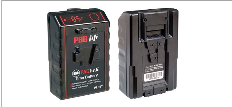
PAGlink batteries are smaller and lighter for their capacity than those of other manufacturers. Individually, PAGlink batteries offer approximately 96 watt-hours capacity (14.8V 6.5Ah). They mount to the camera via the Sony V-Mount connector. Three linked PAGlink batteries, weighing less than 2.2kg, create a single power source of 288 watt-hours (more than four and a half hours run-time for a camera that consumes 60W).
