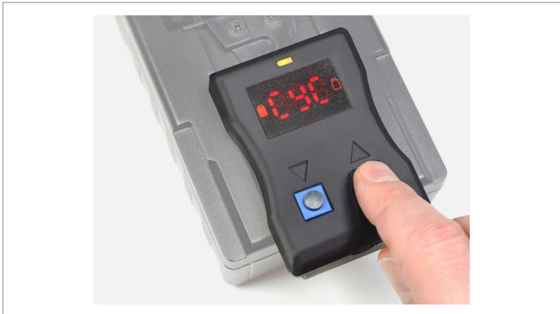
A PAGlink Battery Reader is available that will read data stored in the battery's microprocessor.
